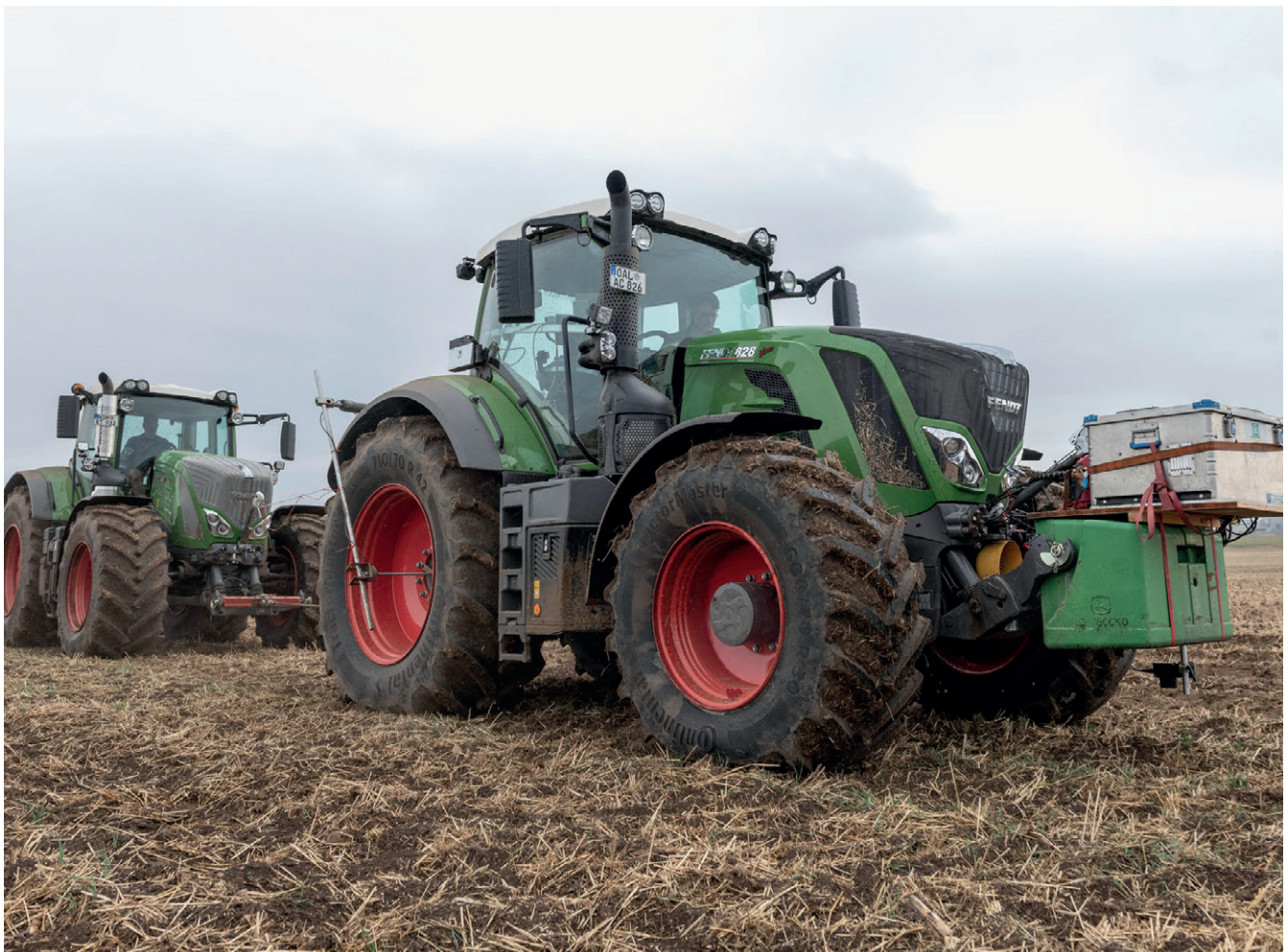
Figure 2: Towing tractor and braking tractor to determine traction and fuel efficiency in a field
