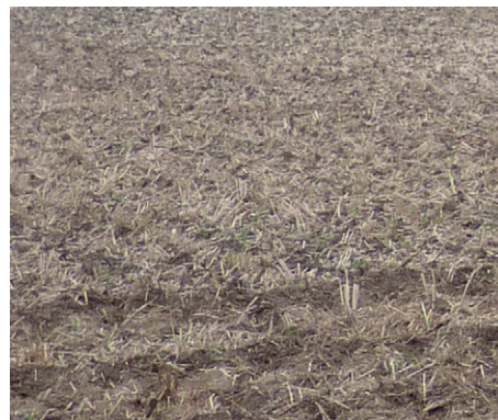
Figure 3: Soil condition at test location (wheat stubble grubbed; black earth consists of loess; middle soil humidity 10% in around 10 cm depth)
