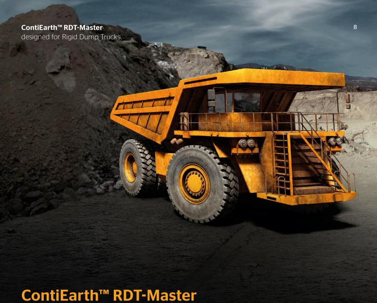
Rigid dump trucks are built to haul heavy loads over long distances in rough terrain. In these severe applications tires have to offer high stability and good traction even at higher speeds. In addition, the tires need to be extremely resistant to cut and tear. The RDT-Master is the perfect fit for transporting extra-heavy loads in adverse condi-
